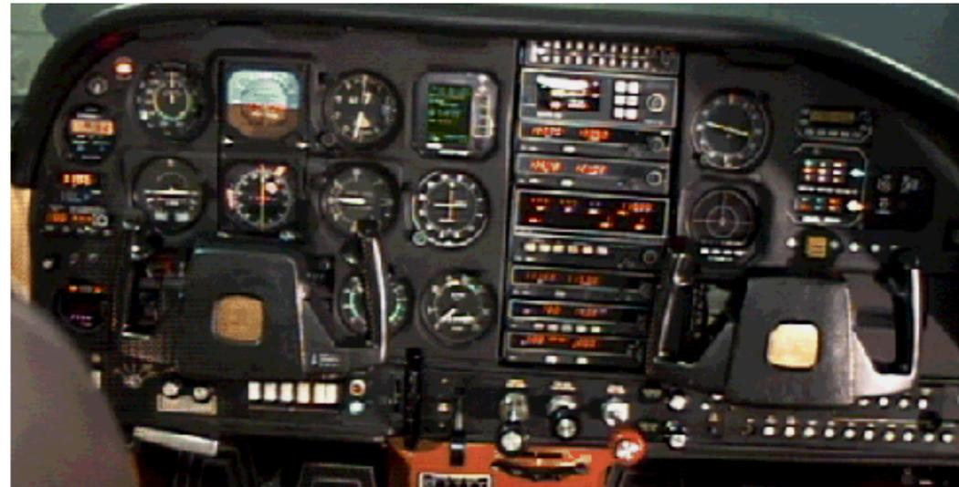
Ready to start? Select 'both' on the left-both-right-off fuel selector, prime with the electric fuel pump and crank with the mixture off. The Lycoming 4-banger is as strong as they come and a predictable starter.
