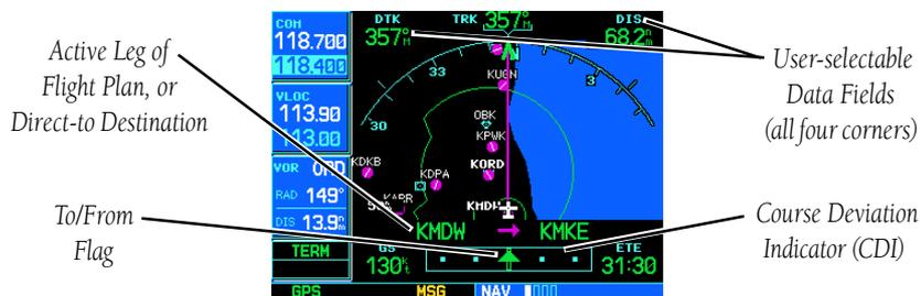
The following symbols are used—directly above the graphic CDI—to depict the “active leg” of a flight plan or direct-to:
