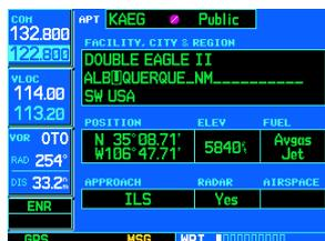
4. Use the **small and large right knobs** to enter the facility name or city location of the desired airport. As you spell the facility name or city, the GNS 530's Spell'N'Find feature will select the first entry in the database based upon the characters you have entered up to that point.
